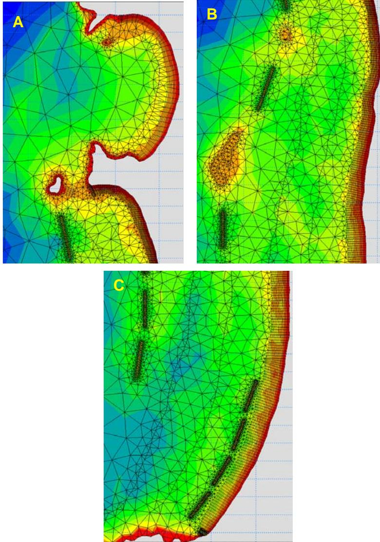
Figure 1 Computational mesh with proposed breakwaters
